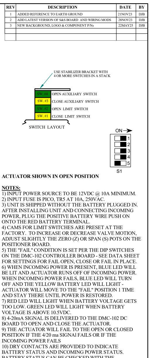
BATTERY STATUS CAN BE CHECKED WITH THE INCOMING POWER ON BY SHORTING THE 2 BATT TEST POINTS J7-2 & J10-1 MOMENTARILY.
