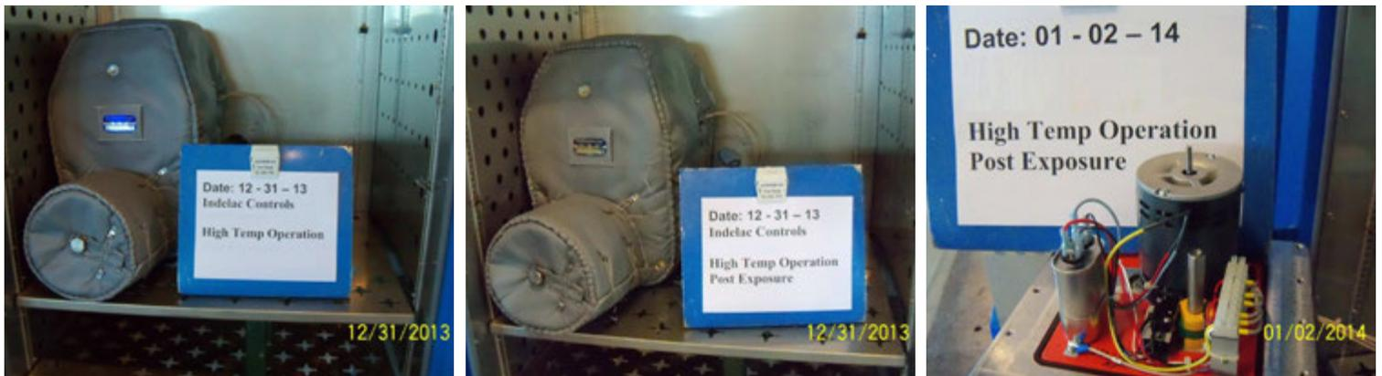
The actuator was installed in an environmental chamber then the temperature inside the chamber was ramped up to 482°F (250°C). The actuator was inside the chamber for duration of two hours and was powered open then closed every ten minutes.
