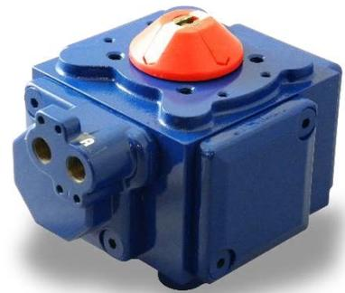
The most practical pneumatic actuators utilize an air pressure supply of 40 to 120 psi (3 to 8 bar). Generally they are sized for a supply pressure of 60 to 80 psi (4 to 6 bar). Higher air pressure is usually difficult to guarantee and lower pressures require a very large diameter piston or diaphragm to generate desirable operating torque.
