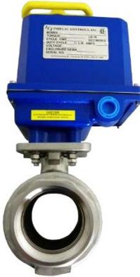
Electric rotary actuators are basically geared motors with a variety of electrical accessories (limit switches, heater, and circuit boards) that may be specified to meet the exact valve automation requirements of a process control system. As an electrical device it is housed in an enclosure designed for specific area classifications (NEMA Rating).
